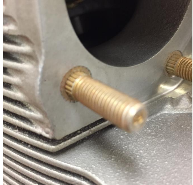
Figure 2 SA638125 Ring Lock Alloy Steel Stud
